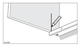
■ At the front edge of the spacer strip draw a vertical line on left and right side of the inside cabinet.
